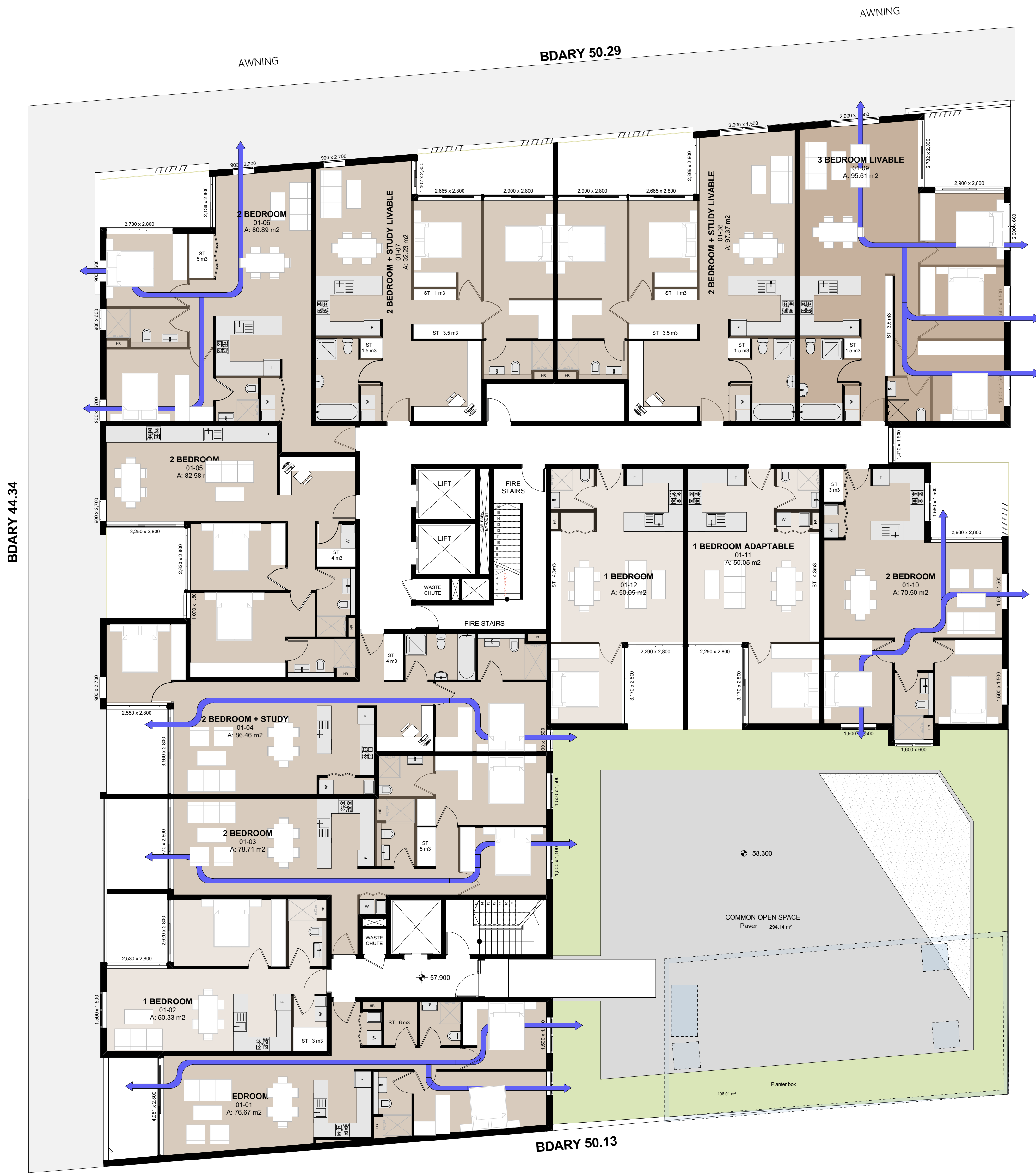
FIRST FLOOR - CROSS VENTILATION DIAGRAM 1:100
