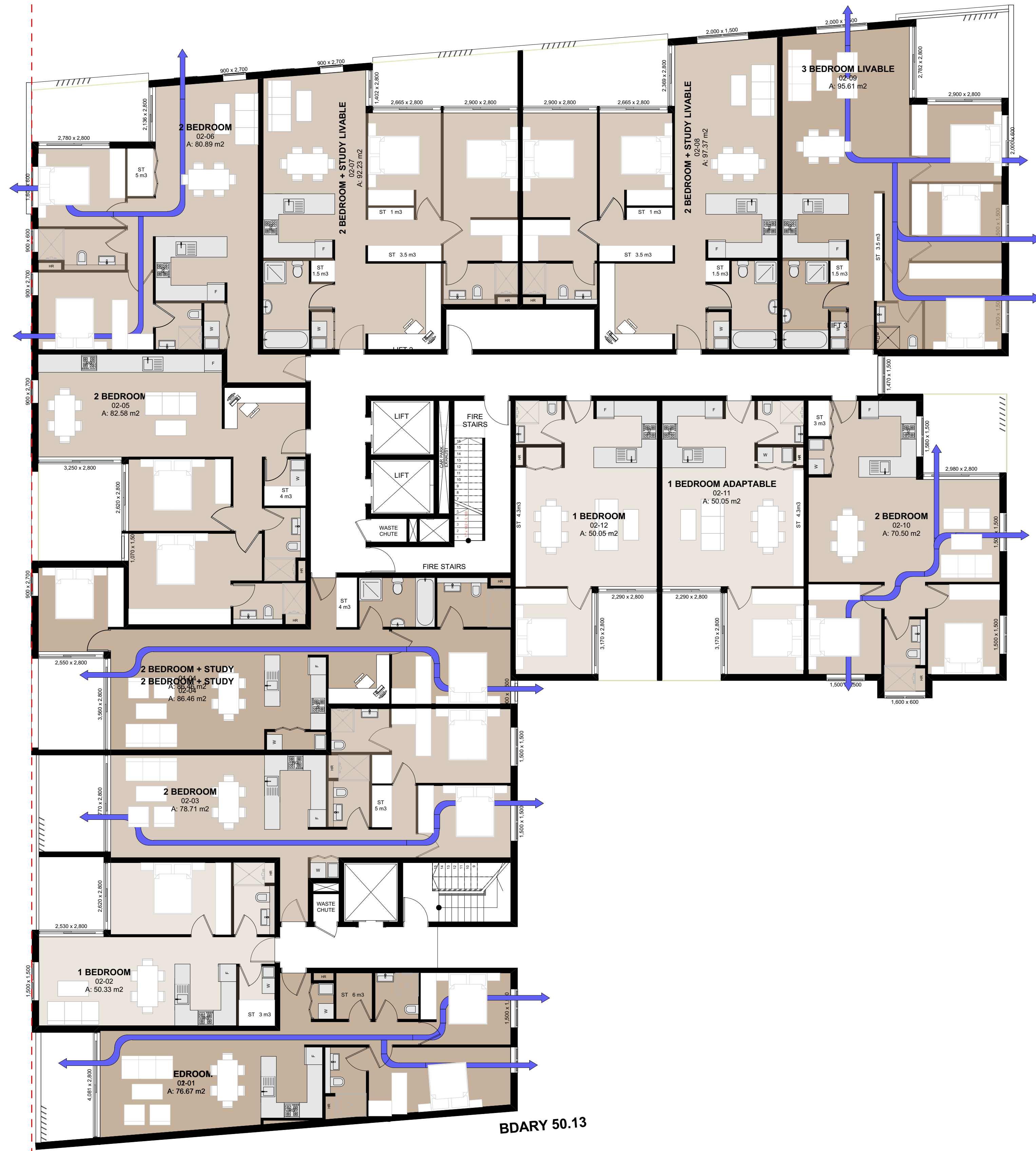
1 SECOND FLOOR - CROSS VENTILATION DIAGRAM 1:100
